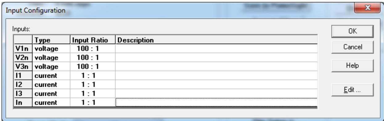
Double click on the input ratio for each voltage input that has a 5KVP attached and enter the input ratio. When done, click on “OK”.
