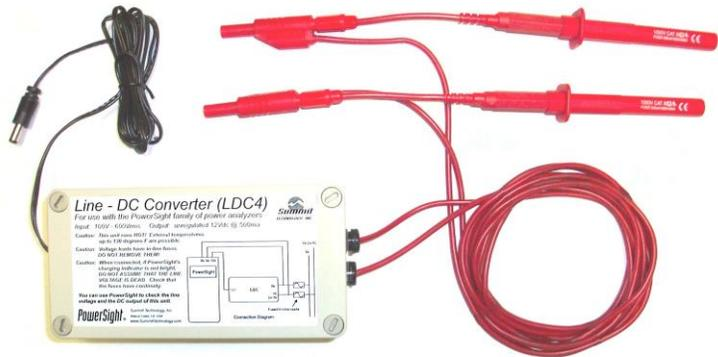
The two inputs of the LDC4 can be freely connected to any two phases or neutral, from 100–600 Vrms, from 50–60 Hz without affecting the output, providing foolproof operation and maximum flexibility. Safety is promoted by fused input leads, insulated grabber jaws, and remote jaw actuators that keep fingers 3 inches away from the hot voltage while attaching the LDC4.
